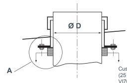
Use spacers between the half collars to allow for future tightening Cushions VI700-A06 (25 mm thick) or VI700-B06 (16 mm thick) Necklace and screw not supplied.
