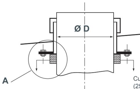
Use spacers between the half collars to allow for future tightening
